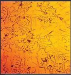
Photomicrograph showing graphite form in gray iron.
