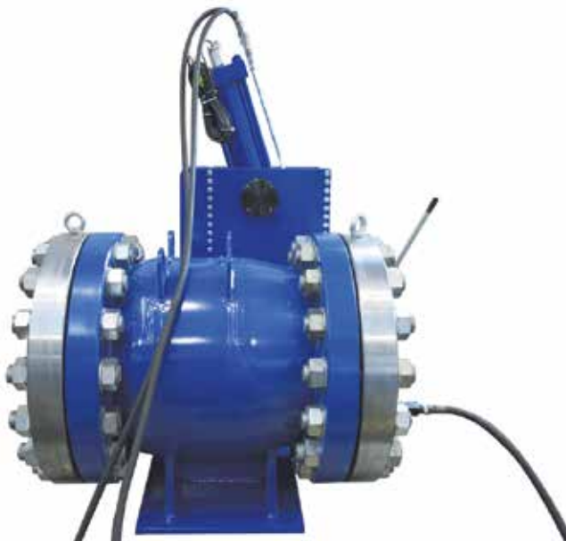
F600 PN100 HYDRAULIC TEST (PRESSURE TEST = 150 BAR)
